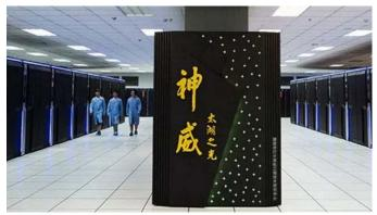
Sunway TaihuLight — As of May 2018 this Chinese computer became the world's fastest. It tripled the speed of China's previous number one super computer, from 33.8 petaflops to 93. That means it can carry out 93 quadrillion calculations per second! To achieve this speed, it has 10,649,600 computing cores. The United States has the third fastest super computer operating at "only" 17.3 petaflops.
